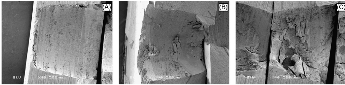
Fig. 2 – SEM images of representative fractures specimens. (A) Adhesive mode of failure: note the scratch lines on dentin, caused by bur action during the cavity preparation procedures. (B) Mixed failure involving adhesive, composite and dentin: the predominant mode of failure in the study. (C) Cohesive failure within the composite: this mode was observed only for specimens activated by soft-start and pulse-delay methods.
